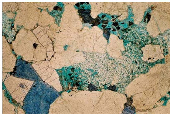
Photomicrograph of a sandstone sample (ppl)
